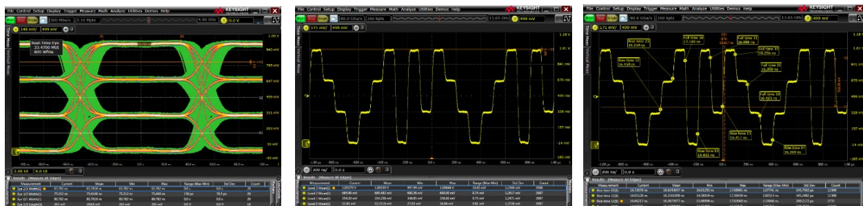
Figure 8. PAM-4 eye, level and rise/fall time measurements.
