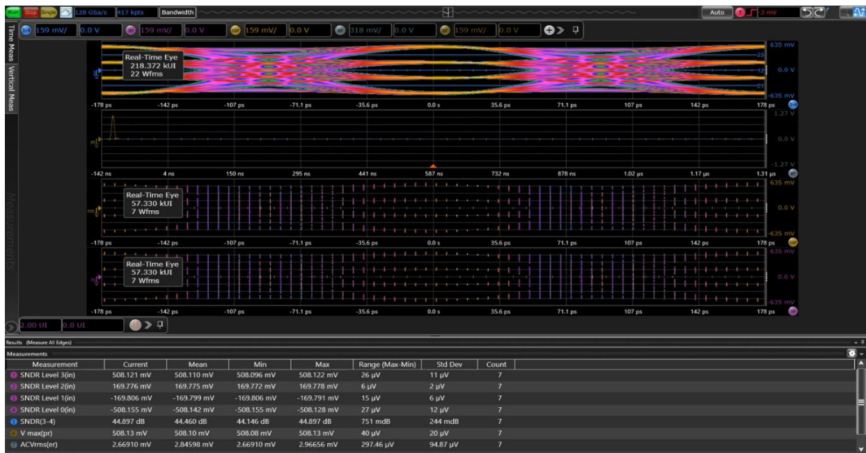
Figure 10. PAM-4 SNDR measurements result
