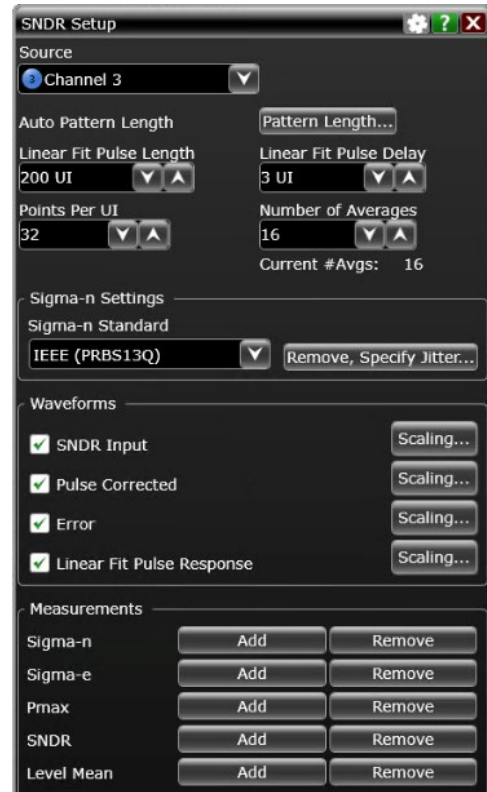
Figure 9. PAM-4 SNDR setup
