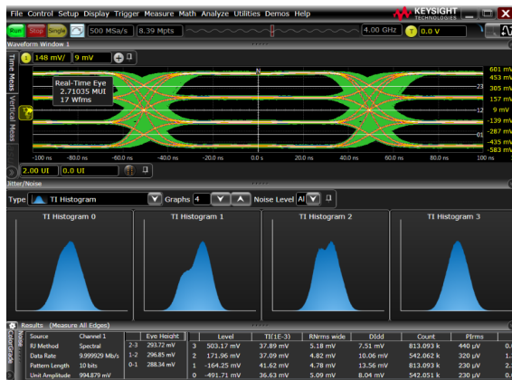
Figure 6. PAM-4 Noise Measurements
