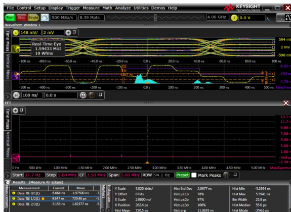
Figure 7. PAM-4 Jitter (Data TIE) Measurements
