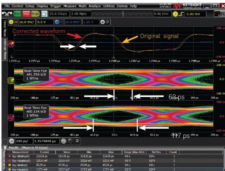
Figure 21. Expanded timebase view of the FPGA serial data with and without the effects of the DC supply noise.
