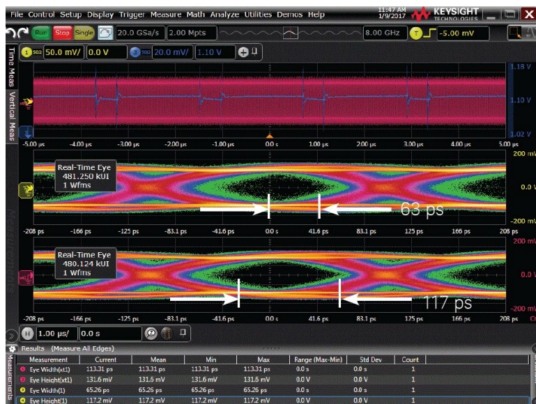
Figure 20. Results from the D9010POWA PI analysis application showing the eye diagram of the FPGA serial data before and after the effects of the DC supply noise are removed.
