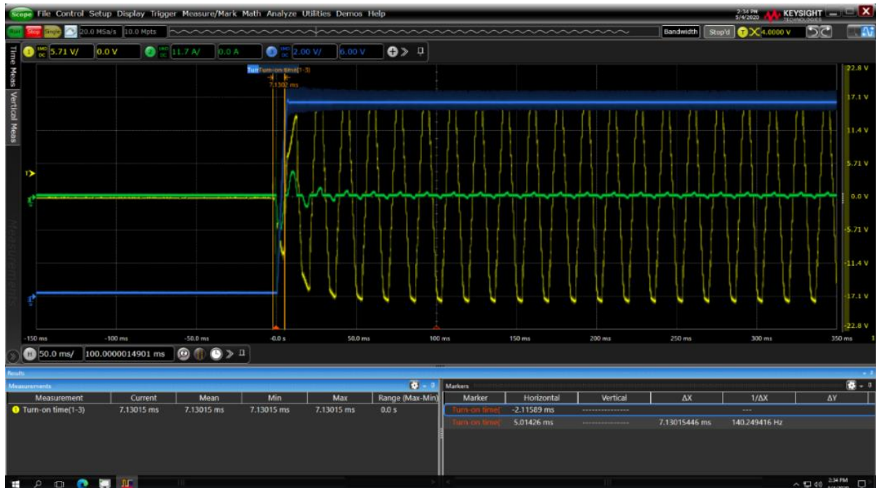
Figure 6. AC-to-DC turn-on time measurement
