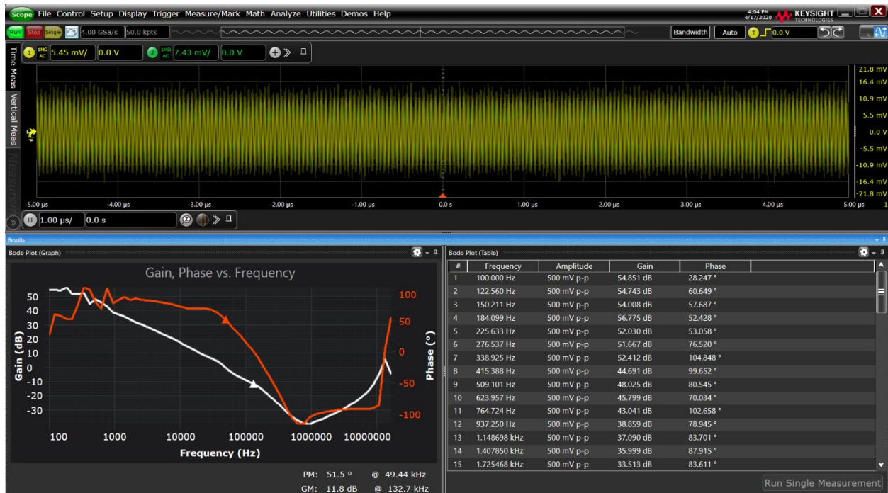
Figure 8. Control loop response measurement with automatic phase margin (PM) and gain margin (GM) measurement
