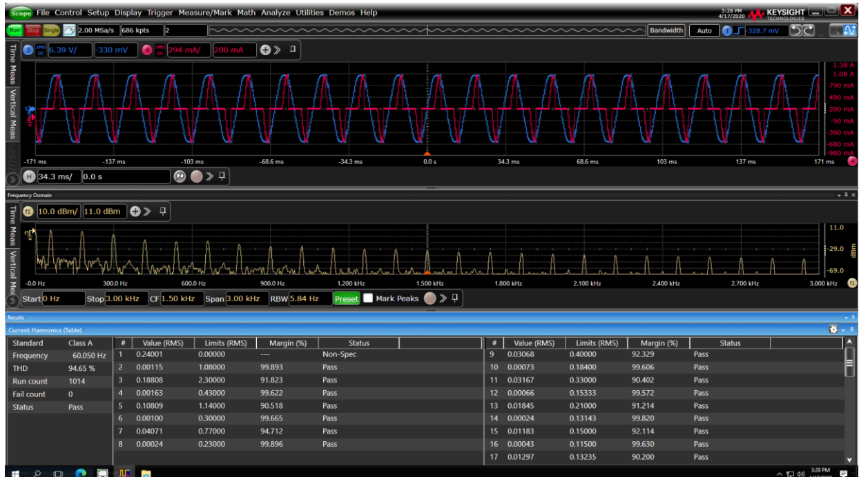
Figure 3. Current harmonics measurement based on IEC 61000-3-2 standards
