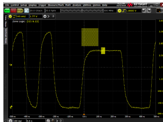
Figure 3. InfiniiScan measurement finder triggers on all edges, then only displays signals with rise times less than 50 or greater than 70 ns
