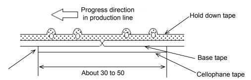
No lifting for the direction of progressing
