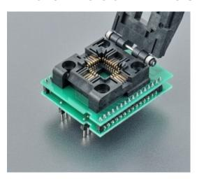
Universal adapter, assigned for devices in PLCC32/LCC32 (for example EPROMs, EEPROMs, FLASHs, Serial FLASHs) support also LCC32 packages
