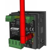
XBEE Wireless transmission via 2,4 GHz mesh network
