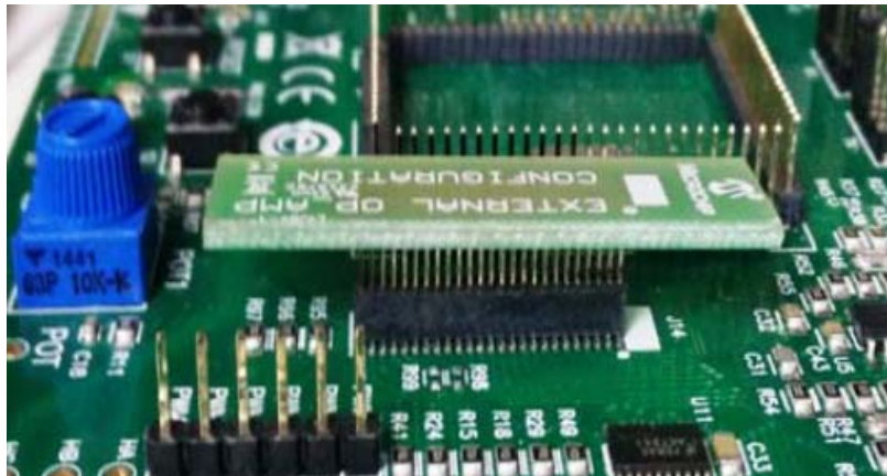
Figure 2. Op amp Configuration Board for dsPICDEM™ MCHV-3
