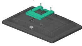
3. Assemble desktop stand to I-series using (4) M4 pan head screws included with stand.
