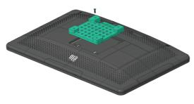
2. Assemble adaptor to I-series using (4) M4 flat head screws (included with kit), in 75mm VESA mounting holes.
