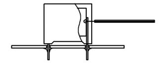
Temperature monitored inside the capacitor.
