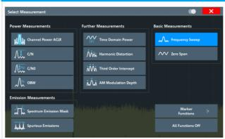
Fast and easy access to a wealth of measurement and marker functions in the base model, including spectrogram measurements and I/Q analysis. Quick configuration through clear menus and touchscreen operation.
