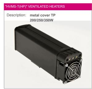
Heating element:PTC thermistor, self regulatingOverheat protectionIntegrated bi-metal thermal protectorHeat sink:black anodised extruded aluminium profile
