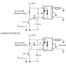
To ensure that the product operates correctly, use the following formula to calculate the limiting resistance, and design the circuit accordingly.
