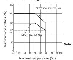
The maximum coil voltage refers to the maximum value in a varying range of operating power voltage, not a continuous voltage.
