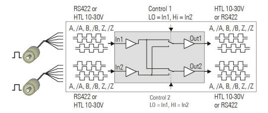
Both inputs can be individually set to either symmetric (differential) format using A, /A, B, /B, Z, /Z channels, or to asymmetric (single-ended) format using A, B, Z channels only. Acceptable input levels are RS422, TTL and HTL 10 ... 30 V.
