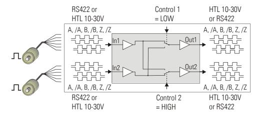
Both inputs can be individually set to either symmetric (differential) format using A, /A, B, /B, Z, /Z channels, or to asymmetric (single-ended) format using A, B, Z channels only. Acceptable input levels are RS422, TTL and HTL 10 ... 30 V.
