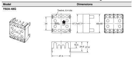
Note: The Terminal Cover can be used with a Back-mounting Socket (P3G-08 or P3GA-11) to create a finger-safe construction.
