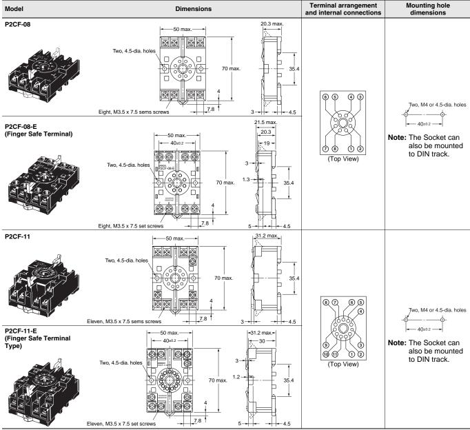
Note: Round crimp terminals cannot be used on Finger-safe Sockets. Use forked crimp terminals.
