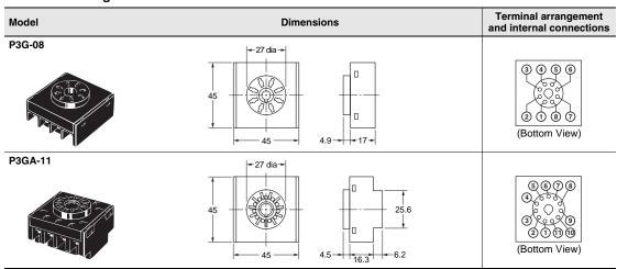
Note: A Y92A-48G Terminal Cover can be used with the Socket to create a finger-safe construction.
