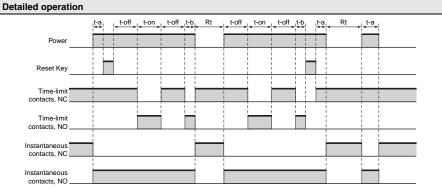
t-on = ON time, t-off = OFF time, Rt = Reset time (0.1 s min.), t-a < t-off and t-b < t-on (Indicates the time is less than the set time.)
