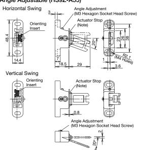
Actuator Mounting Hole Layout (horizontal/vertical swing)
