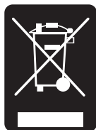
Fig. 1.4: Product labeling in accordance with EN 50419.
