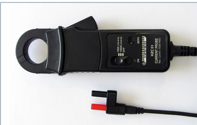
Fig. 4.9: HZC51 Clamp-on current probe.
