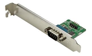
The ICUSB232INT1 USB to RS232 Serial Adapter lets you add an RS232 port to any desktop system that is equipped with an available USB motherboard header.
