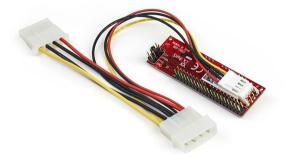
The IDE2SAT2 40-pin IDE to SATA adapter enables you to connect a SATA I/II/III drive to an available IDE/ATA 33/66/100/133 motherboard port - a cost effective solution that allows you to add newer SATA drives, and keep your existing motherboard.
