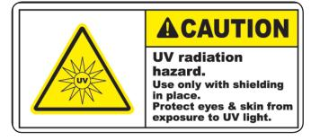
These products generate UVC radiation which can cause skin damage and conjunctivitis to humans and animals within a short time. The skin and eyes must be fully protected against exposure. You should be aware that UVC radiation does not eliminate harmful non-degradable substances such as heavy metals or pesticides. Assume IEC62471 Risk Group 3
