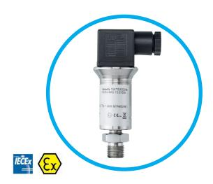
The IPSLAT series is ideally suited or use in a wide range of industrial applications in hazardous areas. The transducer uses a piezo-resistive silicon sensor in a stainless steel housing giving excellent media compatibility for the harshest of applications.
