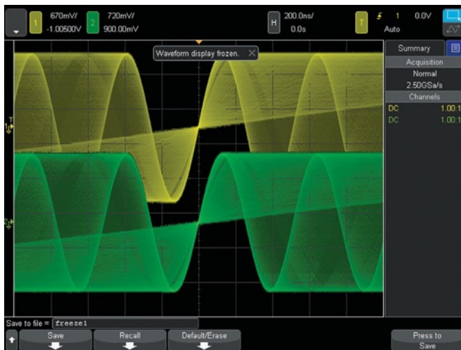
Figure 42. The “freeze screen” feature keeps the intensity-grading information while stopping the waveform acquisition.
