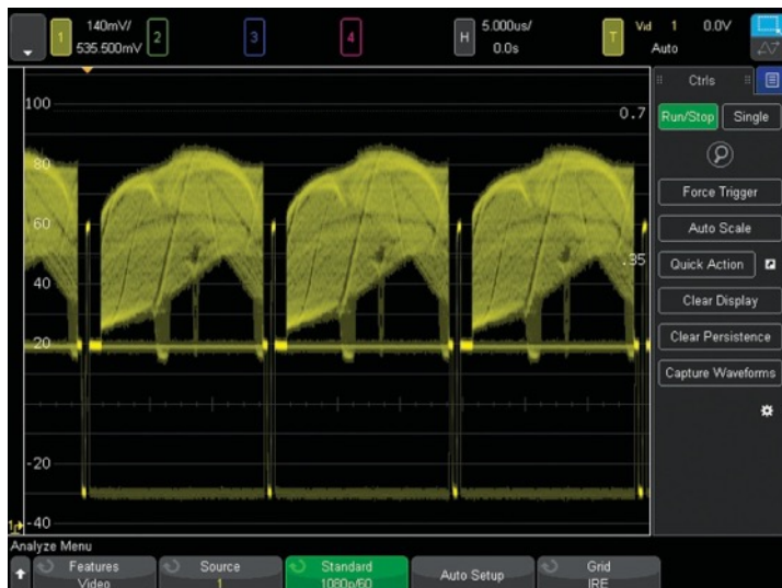
Figure 27. Triggering on 1080p HDTV signal analysis.
