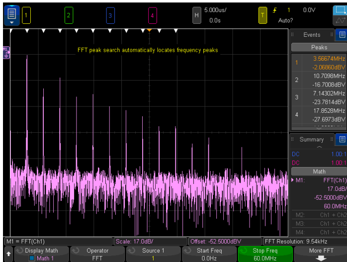
Figure 10b. The 4000 X-Series was set up to capture clock signals for FFT analysis. Using the search and navigation capability, the scope found, marked (white triangles) and quickly navigated to the first 11 frequency peaks occurrences. You can sort it in the order of frequency or amplitude.
