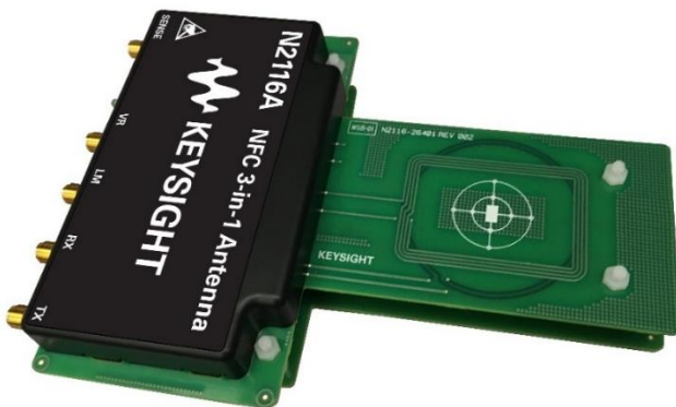
Keysight's N2116A 3-in-1 programmable NFC reference antenna.
