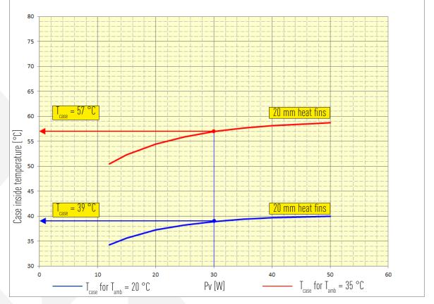
Tested with Mini-ITX Board Core I7 Processor 4770.
