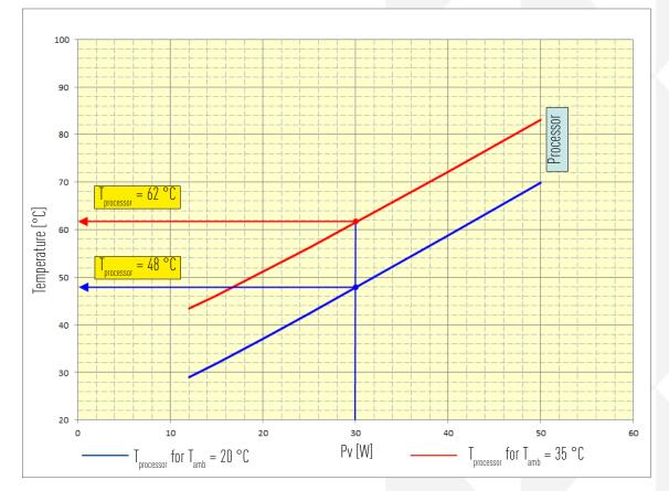
Tested with Mini-ITX Board Core I7 Processor 4770.
