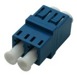
Our range of LC adapters have high precision alignment sleeves for improved reliability and better reconnectability. The LC adapters come with ceramic sleeves for both single mode and multimode. The housing is available in different colors with options for flange or flangeless body and metal or inbuilt clips.
