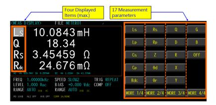
LCR-8200A allows users to select and arrange measurement parameters. Users can select at least one parameter to maximum four parameters from the 17 measurement parameters according to the measurement requirements and the presentation order can also be arranged in a desired manner. The set parameters can be stored in internal/external memory groups for subsequent recalls.
