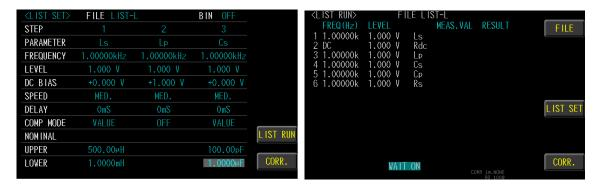
The 15-point LIST measurement mode provides measurement values at a specific frequency or voltage of the DUT, and each set point can set independent comparison and judgement. When the trigger mode is set to "AUTO", the display "WAIT ON" will appear on the measurement screen and LCR-8200A will detect the contact status of the fixture. When the DUT is connected, the test will start automatically.
