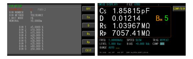
BIN settings for one specific parameter of the selected measurement parameters provide up to 9 BIN positions. Set the judgment basis for individual classifications according to the desired BIN methods (EQUAL/SEQUENTIAL/TOLERANCE/RANDOM) and limit value mode (VALUE/delta/delta%). The result of this sorting can be obtained through the Handler interface. If directly connected to an external device such as a sorter, an immediate sorting can be performed.
