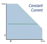
Constant current mode is used for load testing of normal voltage-source power supplies and for constant current discharge testing of batteries.
