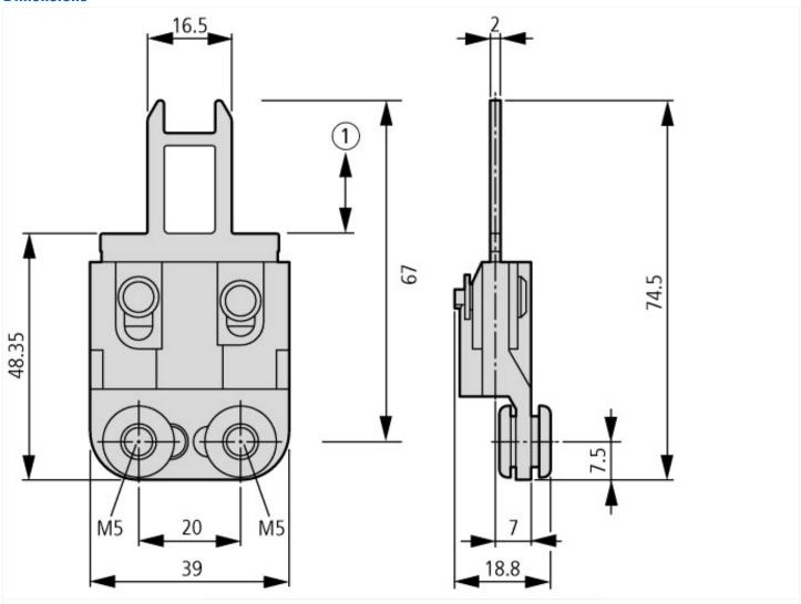
Fixing only allowed with M5 fixing screw and washer according to DIN EN ISO 7093 1 Distance to device head = 0.1  $\dots$  3.0 mm
