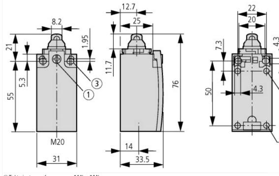
Tightening torque of cover screws: 0.8 Nm ±0.2 Nm
