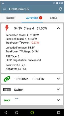
**Link Speed/Duplex** - verify link speed and duplex is configured as expected. If 1000BASE-T test is enabled and the link under test is not performing as expected, a yellow warning indication will be noted and the actual speed emphasized.
