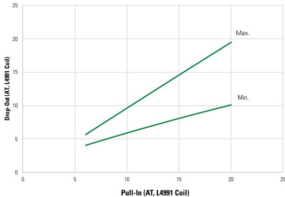
**Note:** The chart represents the range of Drop-Out, minimum to maximum for a given Pull-In value.
