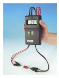
This instrument is a portable digital meter to measure low resistances over the range  $0.001\Omega$  to  $200\Omega$ . A high degree of accuracy is achieved by utilising a four terminal input to eliminate errors caused by test lead length.
