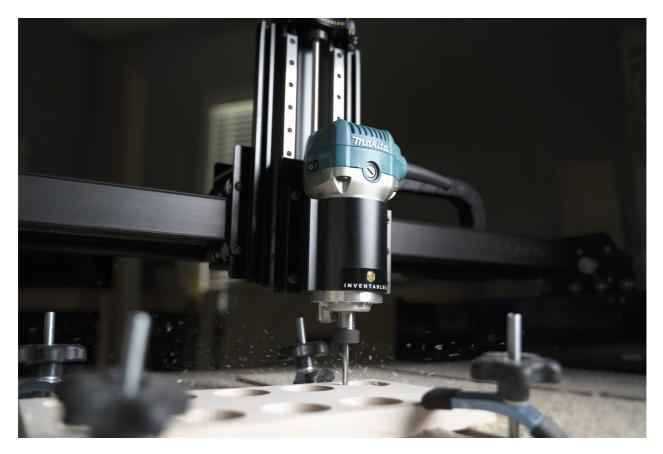
Due to the integrated automatic leveling function, a very well adjusted X-Carve CNC
