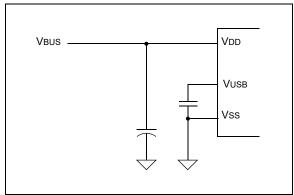
In order to meet the inrush current requirements of the USB 2.0 specifications, the total effective capacitance appearing across VBUS and ground must be no more than 10  $\mu$ F. If it is more than 10  $\mu$ F, some kind of inrush limiting is required. For more details on Inrush Current Limiting, search for that subject in the latest "Universal Serial Bus Specification".
