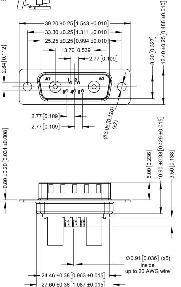
\* UNLESS OTHERWISE SPECIFIED TOLERANCES ON DECIMAL IS: UNIT: MM UNIT: INCH  $X.X \pm 0.25$  $X.X \pm 0.010$  $X.XX \pm 0.13$
