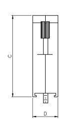
DIMENSIONS(mm/in) В С D А (±0.50) MM  $(\pm 0.50)$  $(\pm 0.50)$ ММ  $(\pm 0.50)$ ΜМ MM SIZE  $(\pm 0.02)$ INCH (±0.02) INCH (±0.02) INCH  $(\pm 0.02)$ INCH ММ MM MM ММ 15.00 31.50 24.99 40.50 9 INCH INCH INCH INCH 1.240 0.984 1.594 0.591 MM 40.00 MM MM 40.50 ММ 15.00 33.32 15 INCH 1.575 INCH INCH 1.594 INCH 0.591 1.312 ΜМ ΜМ MM 54.00 MM 49.50 15.00 47.04 25 INCH INCH INCH 2.126 INCH 1.949 0.591 1.852 MM 70.50 MM MM 54.50 ΜМ 16.00 63.50 37
