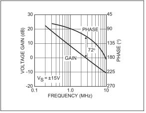
FIGURE 2-6: Gain and Phase vs. Frequency.
