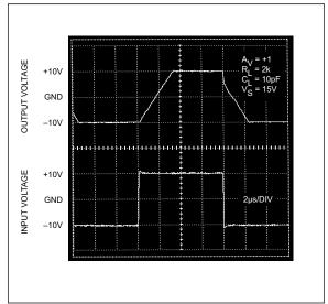
FIGURE 2-11: Large-Signal Transient Response.
