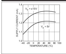
**FIGURE 2-1:** Supply Current vs. Temperature.
