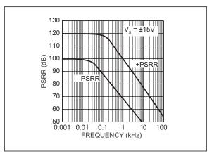
FIGURE 2-9: Power Supply Rejection Ratio vs. Frequency.
