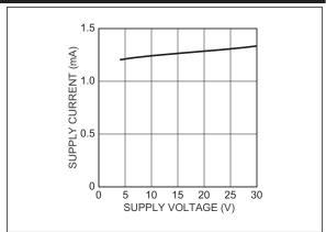
FIGURE 2-4: Supply Current vs. Supply Voltage.
