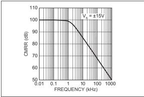
FIGURE 2-8: Ratio vs. Frequency.
