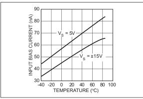
**FIGURE 2-2:** Input Bias Current vs. Temperature.
