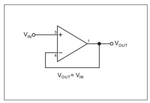
FIGURE 4-1: Voltage Buffer.
