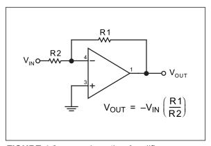
FIGURE 4-2: Inverting Amplifier.
