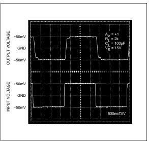
FIGURE 2-12: Small-Signal Transient Response.
