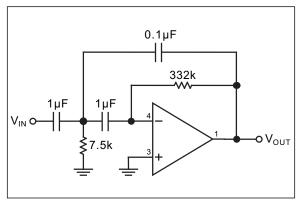
FIGURE 4-4: High—Pass Filter.
