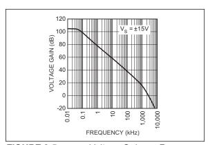
FIGURE 2-5: Voltage Gain vs. Frequency.
