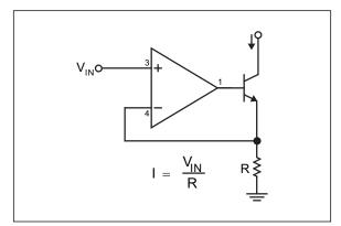
FIGURE 4-3: Voltage Controlled Current Sink.
