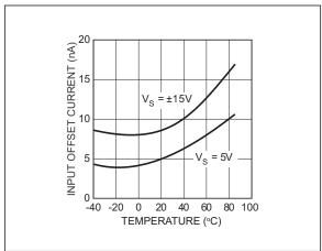
FIGURE 2-3: Input Offset Current vs. Temperature.
