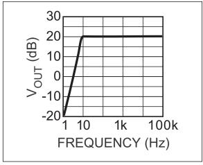
FIGURE 4-5: High-Pass Filter Response.
