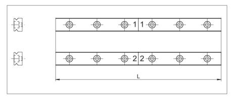
Multi-part guideways are numbered at the butt joint
