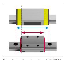
The carriage length remains unchanged with LUBE-S
