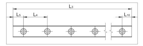
$L_3$  = standard rail lengths in mm  $L_4$ ,  $L_5$ ,  $L_{10}$  = standard hole spacings in mm
