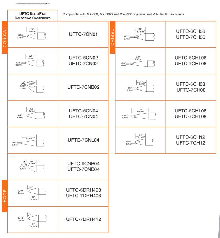
7 = 700 Series for most standard applications 6 = 600 Series for temperature sensitive applications
