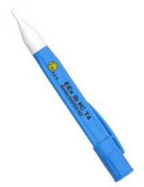
The EEx approved Magnet Stick is an instrument for testing for the presence of magnetic fields. By simply holding the tip of the instrument near the test area, it indicates a magnetic field by glowing. The test lamp responds to all kinds of magnetic fields, from alternating current to direct current and permanent magnets. (Sensitivity 300 gauss 0,3 mT). The ATEX and IECEx approvals are confirmed by NEMKO. (II 2G EEx ib IIC T4) **General Features:**
