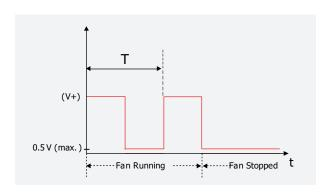
**Tacho Frequency** RPM=60/2T=30 f (f=frequency)
