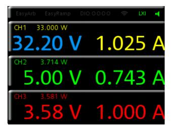
The different operating conditions are marked by colors: constant voltage operation is indicated in green, constant current operation in red, inactive channels are shown in yellow, blue indicates that the channel is in setting mode.
