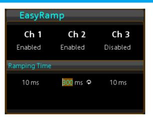
EasyRamp simulates operating conditions with controlled rise of supply voltage to prevent a sudden voltage surge.
