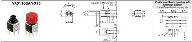
Areas marked 💹 indicate locations of the product's metal parts (bracket). These should be taken into account when designing the circuit board pattern.
