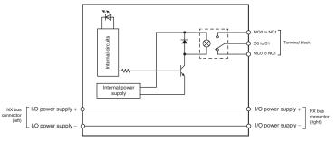
NO0 and NO1 are normal open contacts, and NC0 and NC1 are normal close contacts. You cannot replace the relay.
