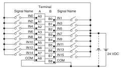
$\bullet$  The polarity of the input power supply can be connected in either direction.
