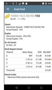
Cabling SNR measurement validates Multi-Gig links
