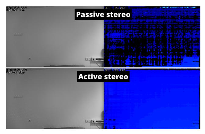
**Flood IR LED** illumination allows perceiving low-light and no-light environments. You can run your AI/CV processes on frames that are illuminated by the IR LED. Note that the color camera doesn't perceive IR light, so you would need to use a mono camera stream for your AI/CV processes.
