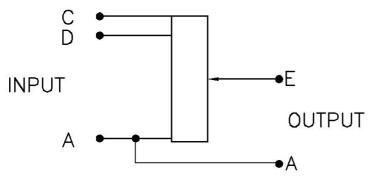
Connection 230V on A - C delivers max. 230V output A - E. Connection 230V on A - D delivers max. 260V output A - E.
