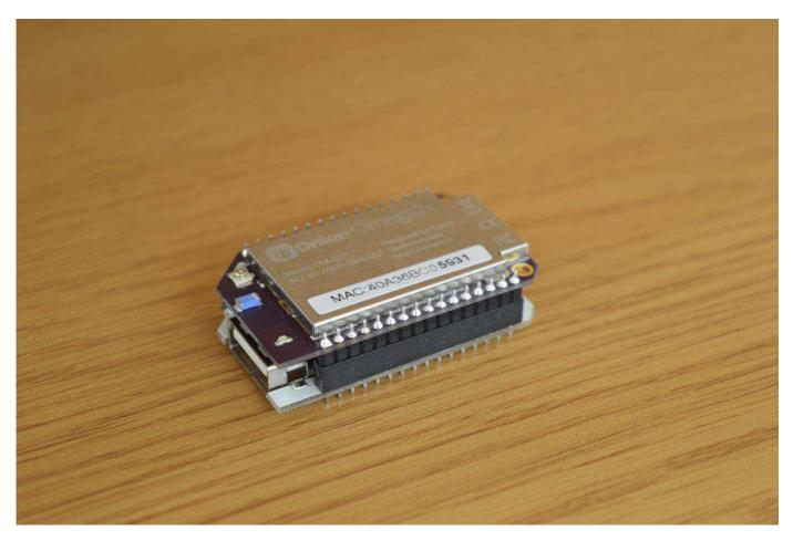
You may need to line up the pins with the holes before pressing the Omega into the Dock.
