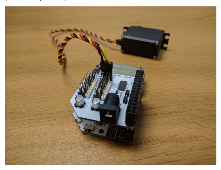
Check out the PWM Expansion hooked up to the servos on our Spiderbot!
