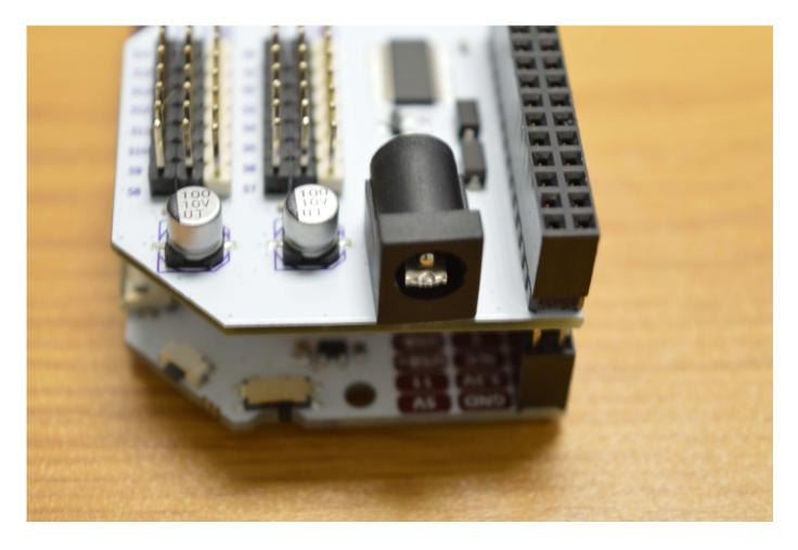
The DC voltage supplied through the barrel jack will be provided on the Vcc (and GND) pins. The PWM voltage will also be stepped up to this voltage.
